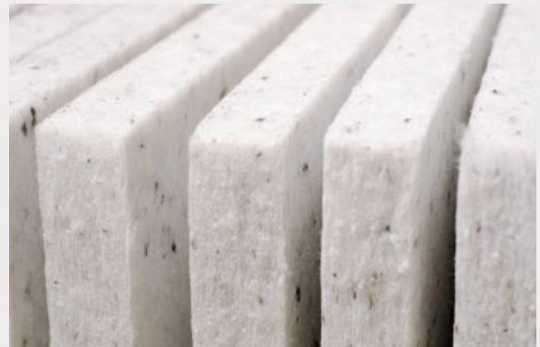
Airlay insulation - randomised fibres
