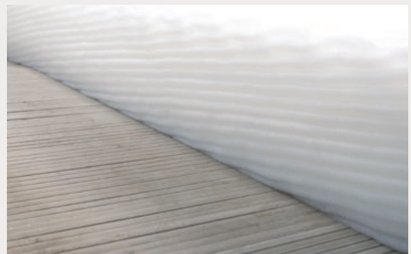
Carded insulation - traditional layering
