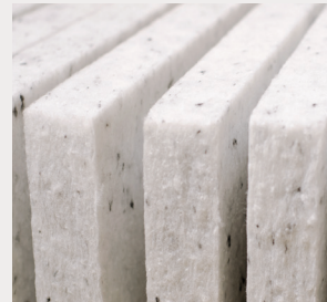
Airlay insulation – randomised fibres
